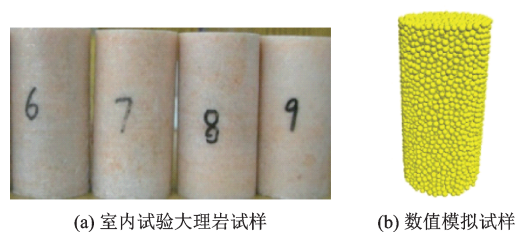
图1 室内试验与数值模拟试样 Fig.1 Laboratory test and numerical simulation samples
